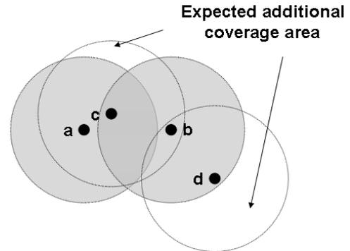
Fig. 1. Example of the expected additional coverage concept
