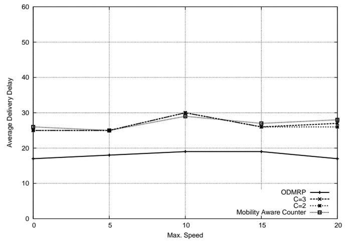
Fig. 13. Average Delivery Delay with 1 source and 15 receivers
