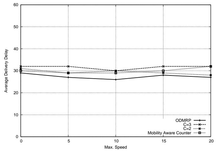
Fig. 14. Average Delivery Delay with 2 sources and 15 receivers
