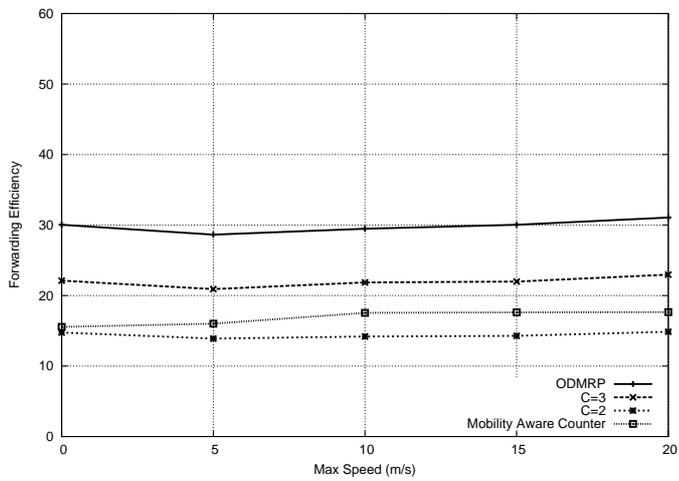
Fig. 10. FEF with 1 source and 15 receivers
