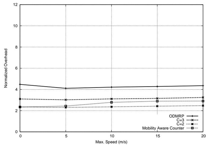
Fig. 8. Overhead with 2 sources and 15 receivers
