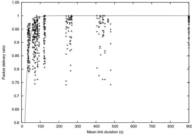
Fig. 3. Packet delivery ratio vs. mean link duration
