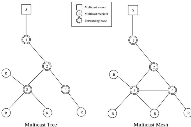
Fig. 1. Tree-based vs. mesh-based multicast forwarding structure
