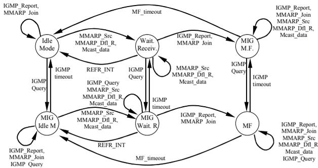
Fig. 6. State diagram illustrating the operation of the MMARP protocol
