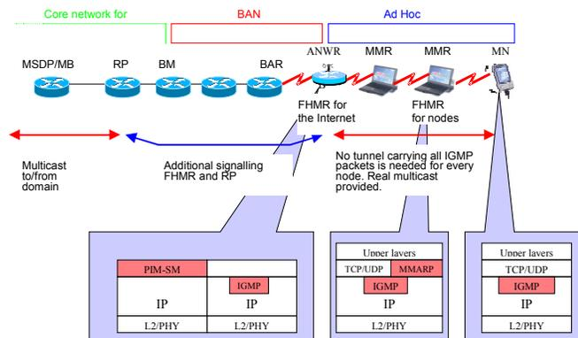
Fig. 2. The proposed MIND architecture with its three constituent parts: the core network, the access network and the ad hoc extension.
