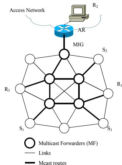
Fig. 5. Example of a MMARP distribution mesh between senders (S) and receivers (R).
