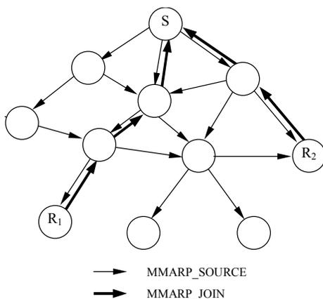
Fig. 4. Two-phases approach for the creation of the multicast distribution mesh in MMARP
