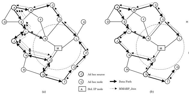
Fig. 7. Two-phases approach for the creation of the multicast distribution mesh in MMARP
