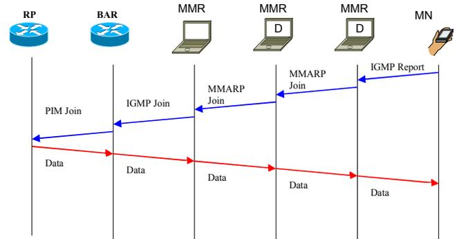
Fig. 3. Example of interaction between the MIND multicast protocols in order to receive a multicast flow
