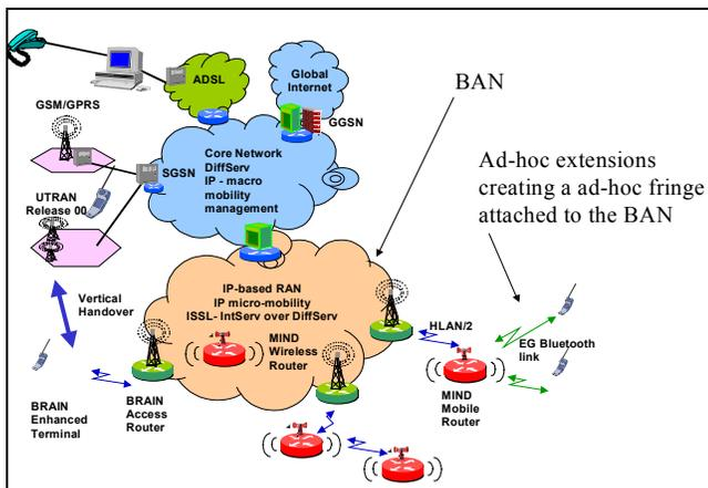
Fig. 1. The MIND reference network architecture consist of three different parts: the core network, the access network and the ad hoc network extension.
