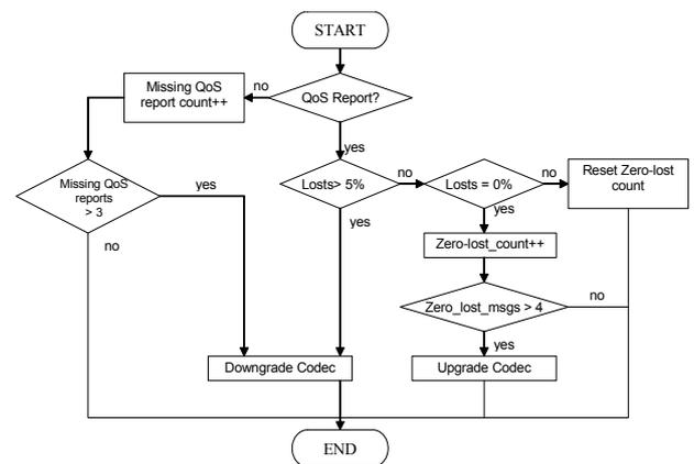
Fig. 3. Schematic diagram of the adaptation logic.
