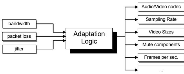
Fig. 2. Operation of the adaptation logic.
