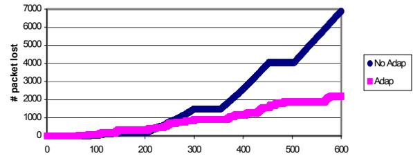
Fig. 6. Packet losses with and without adaptation.
