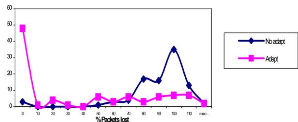
Fig. 8. Packet loss distribution with high interference.
