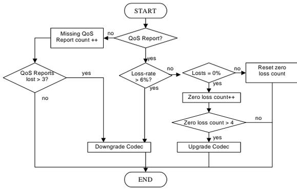
Fig. 2. Diagram of the adaptation logic
