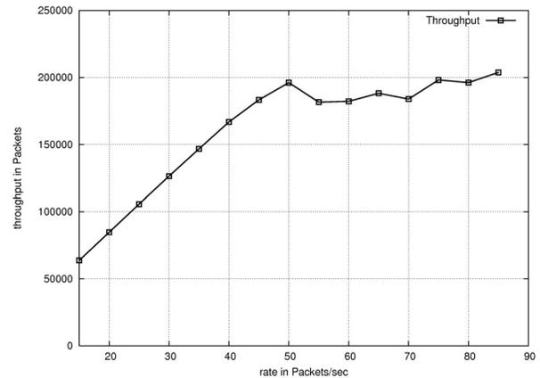
Figure 1: Throughput as function of offered traffic load
