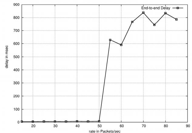
Figure 2: End-to-End Delay as function of traffic load
