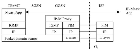
**Figure 4: UMTS configuration for IP Multicast**
