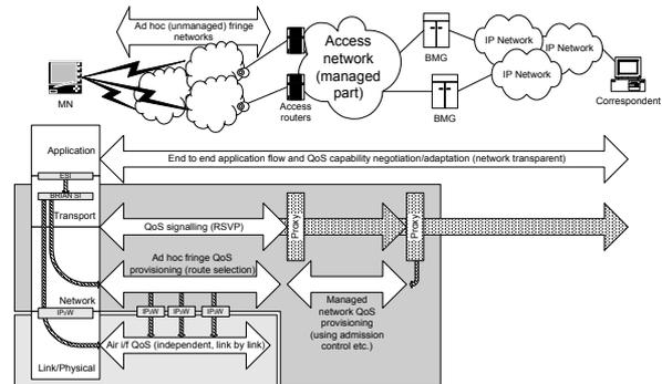
**Figure 2: QoS Provisioning Architecture**
