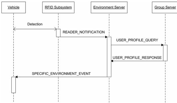
Fig. 4. High level communication architecture
