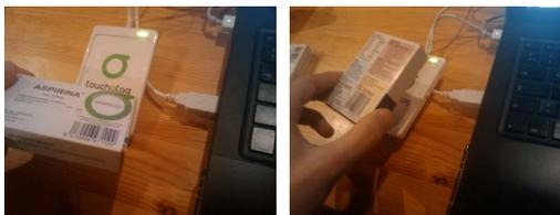
Fig. 6. Identifying drugs using a NFC USB reader.
