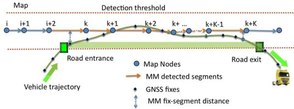
Fig. 2. Correct operation of map-matching using point-segment distance.
