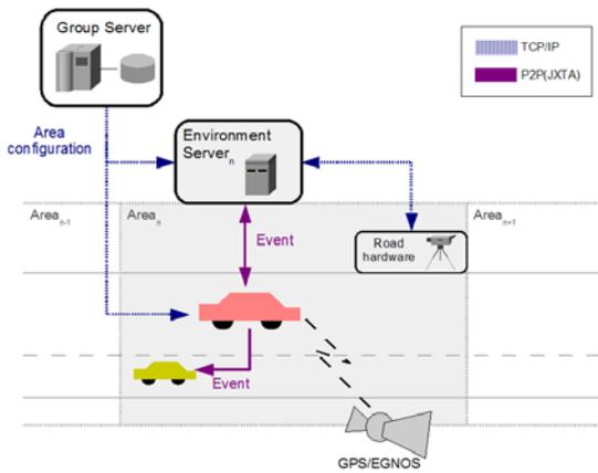
Fig. 3. Overlay vehicular network used in the system.
