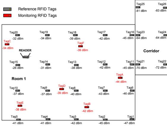
Figure 2. RSSI values obtained from the RFID reader point of view
