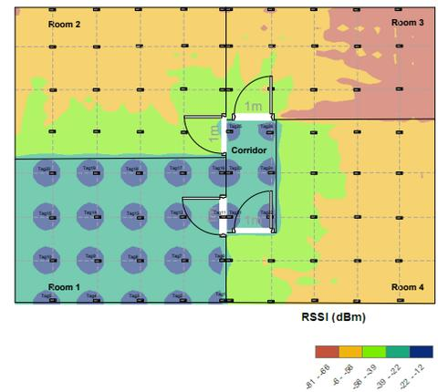
(b) RFID power distribution considering geometrical optics and uniform theory of diffraction.
